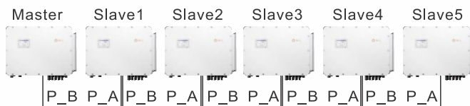
Figure 3.18 Parallel Terminal Connection
