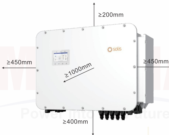
Figure 3.3 Inverter Mounting Clearances
