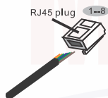
Figure 3.16 Strip the insulation layer and connect to RJ45 plug
