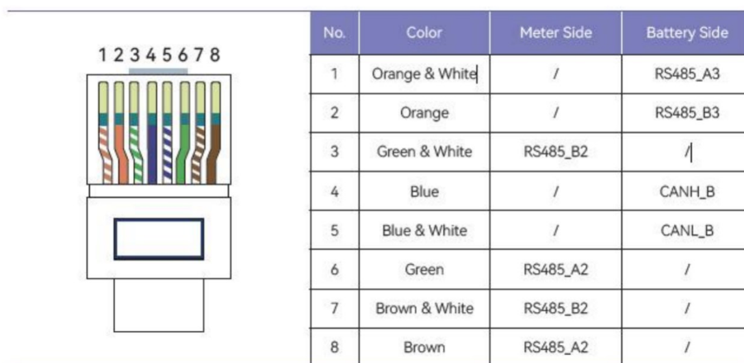
Figure 4.6-1 Hybrid Inverter Communication terminal definition diagram
