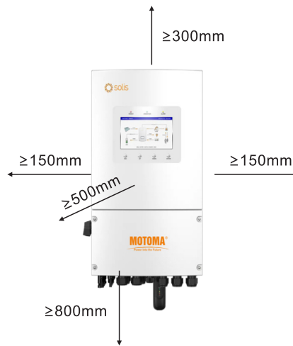
Figure 3.5 Inverter Mounting Clearances
